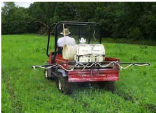
Tractor or ATV mounted herbicide sprayer
